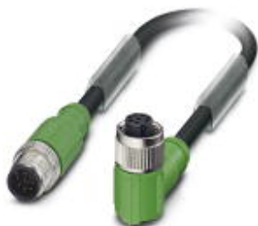
Sensor/actuator cable, 8-position, Variable cable type, shielded, Plug straight M12, A-coded, on Socket angled M12, A-coded, cable length: Free input (0.2 ... 40.0 m)
