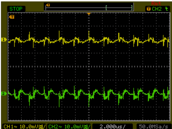
Figure 53: AXA00AA18-L Ripple and Noise Measurement Vin = 24Vdc Load: Io = ±1 A Ch 1: Vo1 Ch2: Vo2
