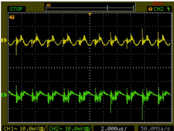
Figure 133: AXA00AA36-L Ripple and Noise Measurement Vin = 48Vdc Load: Io = ±1 A Ch 1: Vo1 Ch 2: Vo2
