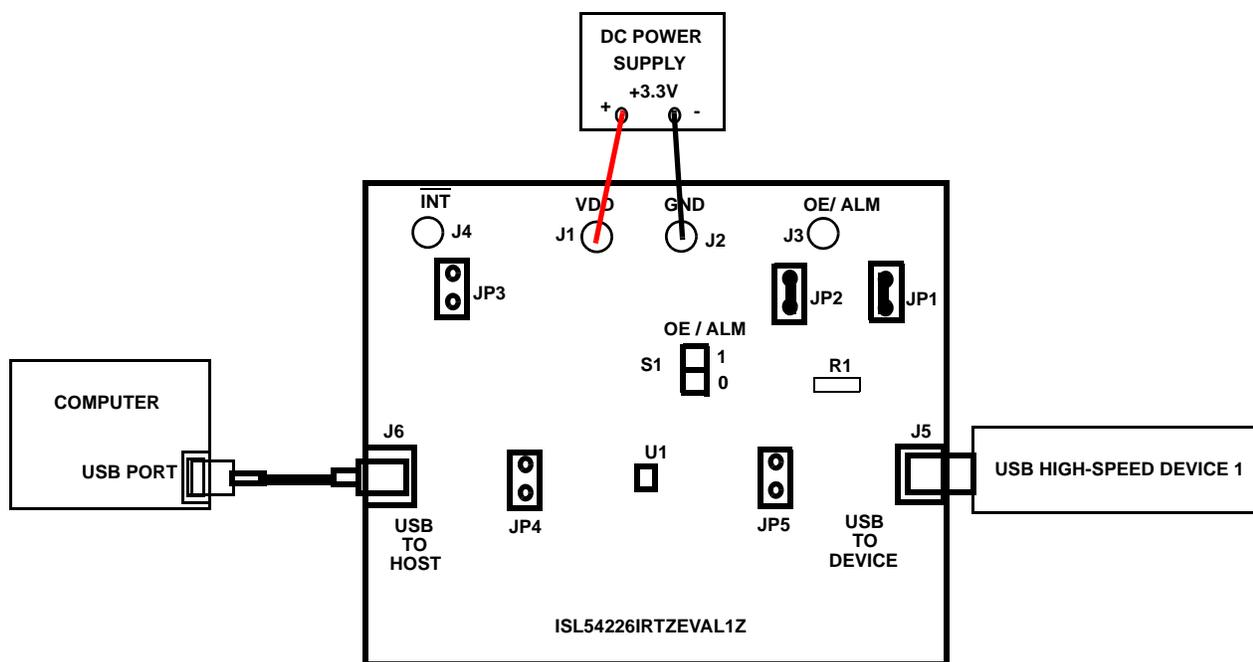
FIGURE 2. BASIC EVALUATION TEST SETUP BLOCK DIAGRAM
