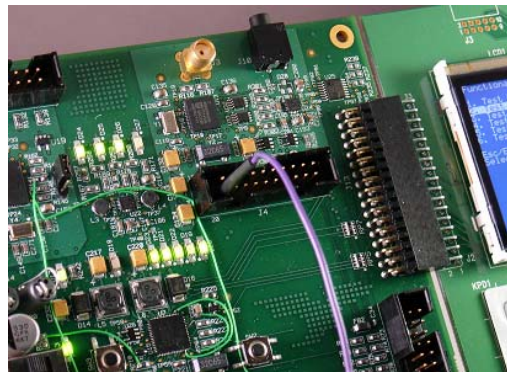
Figure 12 Oscilloscope Ground Connection
