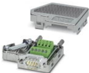
D-SUB connector, 9-pos., male connector, two cable entries < 35°, universal type for all systems, pin assignment: 1, 2, 3, 4, 5, 6, 7, 8, 9 to one screw connection terminal block
