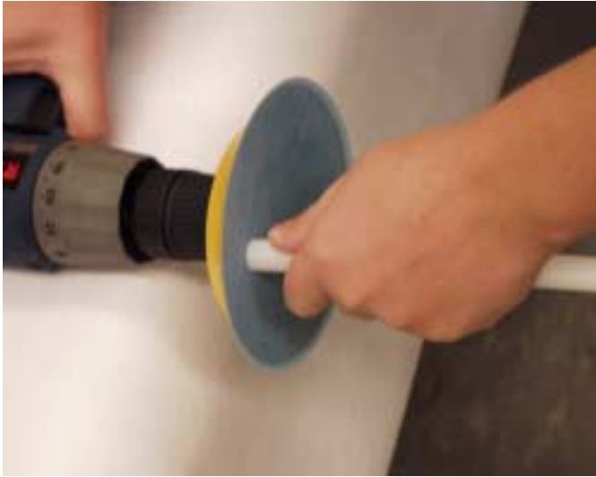
Figure 2. Portable drill used to polish 3M™ Light Fiber
