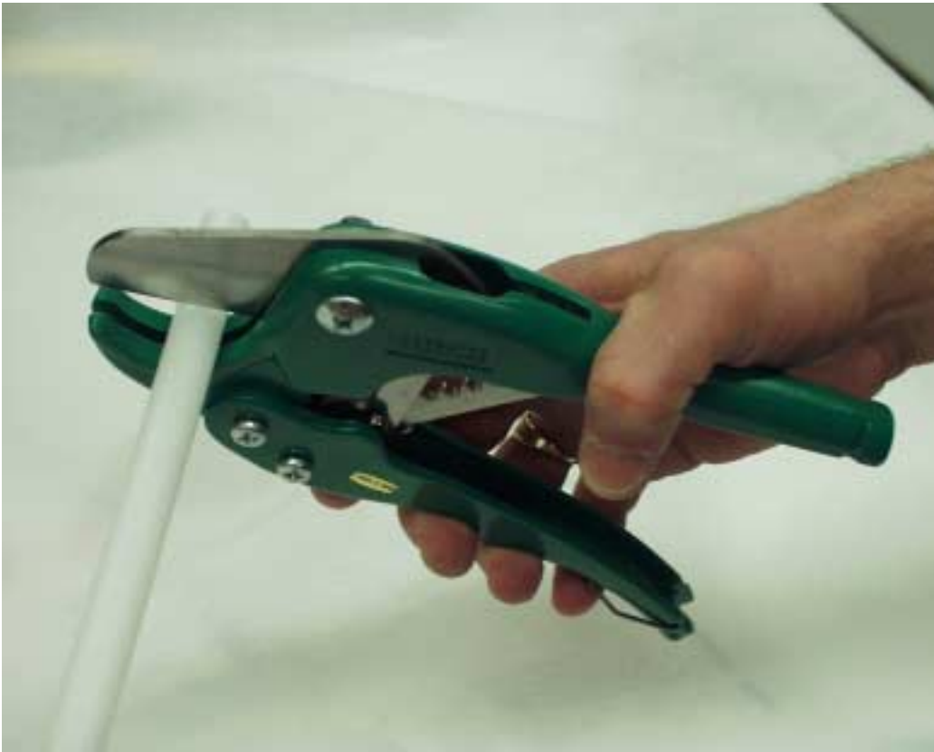
Figure 1. Cutting 3M™ Light Fiber
