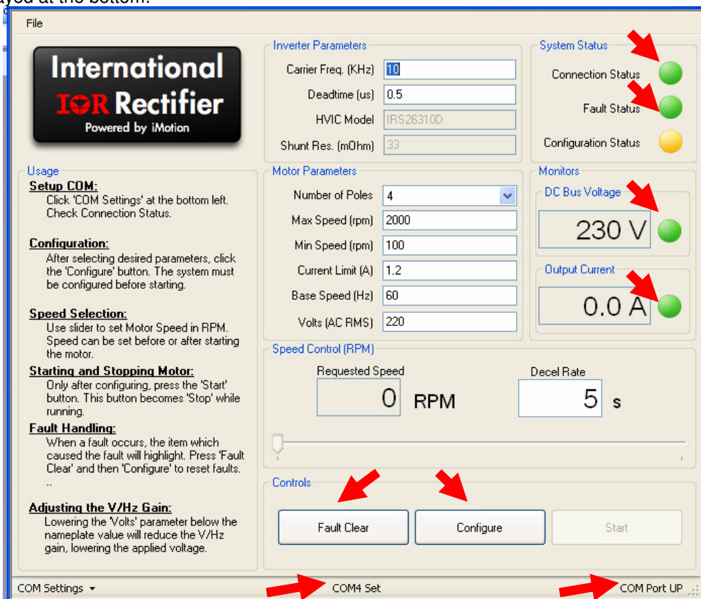
Figure 14: Software GUI after establishing communication between PC & IRMD26310DJ
