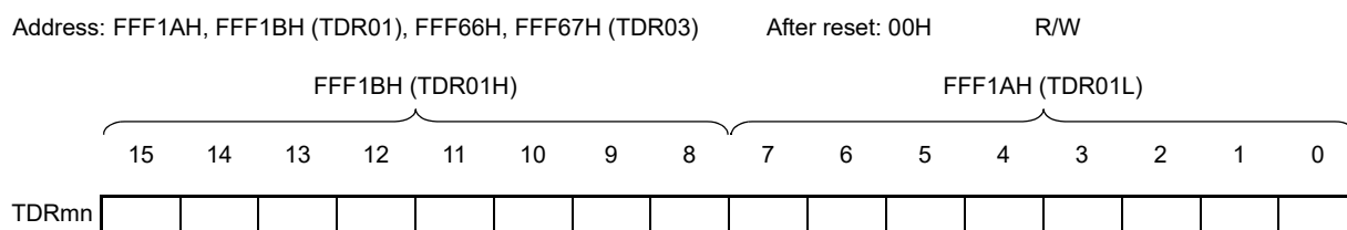
Figure 7 - 8 Format of Timer data register mn (TDRmn) (n = 1, 3)
