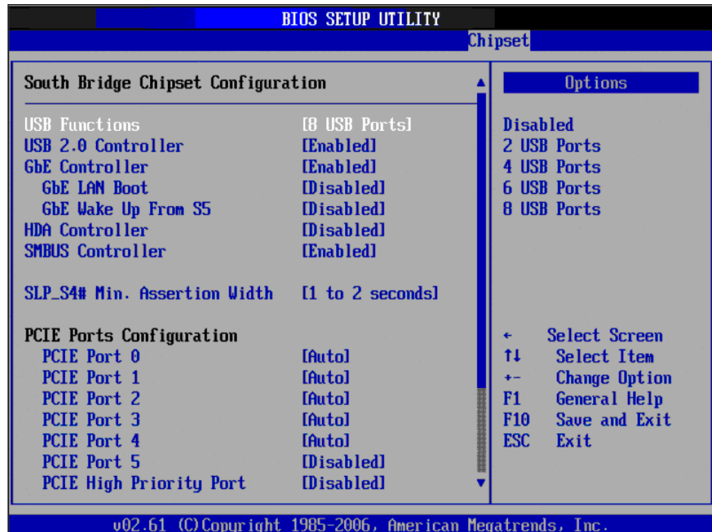
Figure 3.26 South Bridge Configuration
