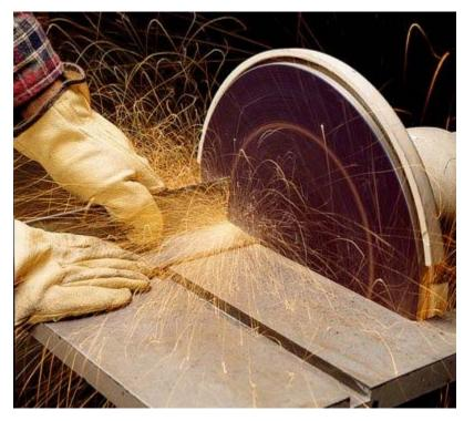
Our 3M<sup>™</sup> PSA Cloth Disc 348D features a heat-resistant resin bond and cloth backing that make this sanding disc a good choice for high heat and heavy duty sanding applications. Aluminum oxide particles in a closed coat offer a fast cut for grinding and dual action (D/A) sanding on metal. This versatile disc provides a fast, efficient method for deburring, blending, cleaning up, and finishing metal parts and surfaces of various sizes and shapes.
